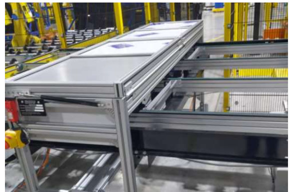
Figure 4. Cameras before the washer in the direction of panel flow
