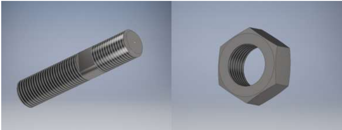
Figure 8. 3D drawing of implant bolts
