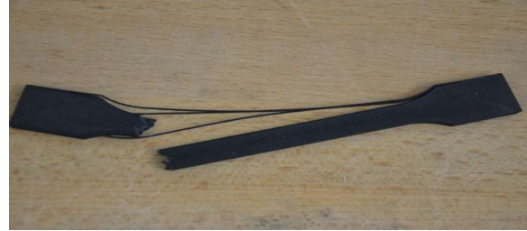
Figure 1. The brittleness and splitting of specimens made by recycled ABS after tensile test.
