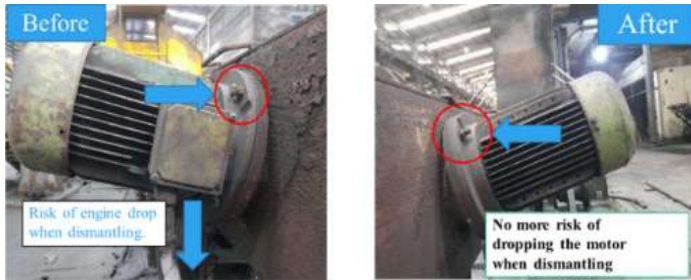
Figure 11. The picture shows that there is no longer a hazard when replacing implant bolts
