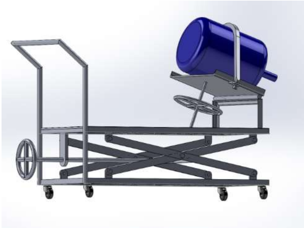
Figure 13. 3D drawing of trolley
