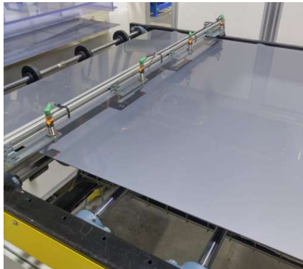
Figure 6. Four sensors capturing the signal
